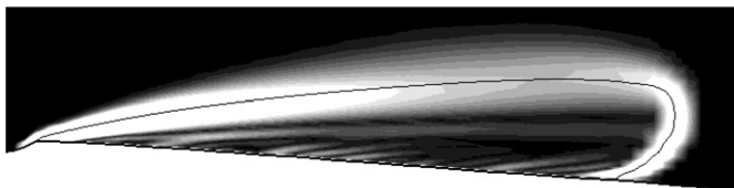
Fig. 20. Magnitude of density gradient ( 0 to 10^6 \text{kg/m}^4 ) and iso-line \alpha = 0.3 L_{\text{sheet}} \sim 80 mm, A_{\text{min}} = 50 .
